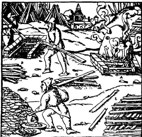
Fig 52 Roasting tin ores (after AGRICOLA, de re Metallica )
