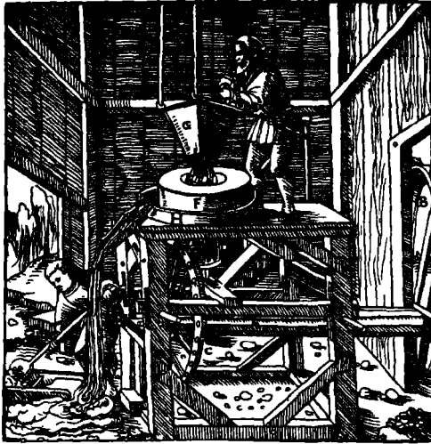
Fig 53 Grinding tin ores (after AGRICOLA, de re Metallica )
