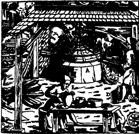
Fig 45 Oxydation of crude lead to produce silver (after AGRICOLA, de re Metallica )
