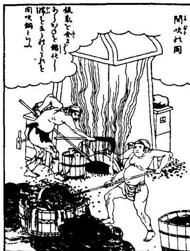
Fig 66 Removing the copper from the smelting furnace (after GOWLAND, Metals )
