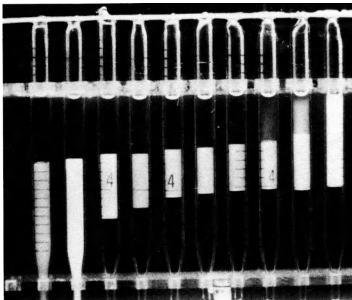
Figure 2. Salinity scan of a sodium sulfonate surfactant, isobutanol, n-hexadecane, and NaCl brine mixture. The surfactant is sodium 4-(1'-heptylnonyl) benzenesulfonate (SHBS). Mixtures were in the volume percent of about 5% surfactant plus alcohol, 45% hydrocarbon and 50% brine. The brine ranged in salinity from about 0.2 to 2 wt% NaCl. Ref. 32.
