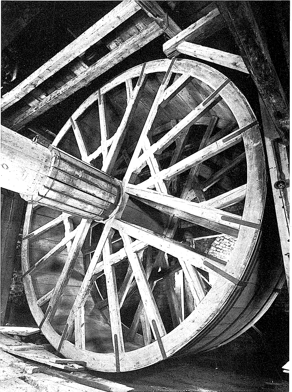
Wooden machines and gears: this enormous tread-mill was a cage operated by three men standing inside. (Lichtbildstelle, Deutsches Museum, Munich.)
