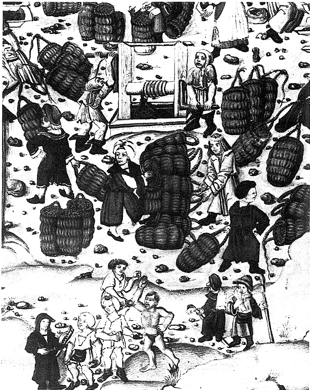
Detail of the silver mine of Kutna Hora, about 1490. The baskets of ore were hauled to the surface by a windlass worked by two men. The same mine possessed giant windlasses worked by horses. But these were still only elementary means. Fifty years later, in the time of Agricola, huge hydraulic wheels were being used for lifting. (Vienna, Aus dem Bildarchiv d. Ost. Nationalbibliothek.)
